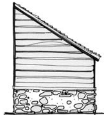
Horizontal Clapboard Siding with Rock Base
