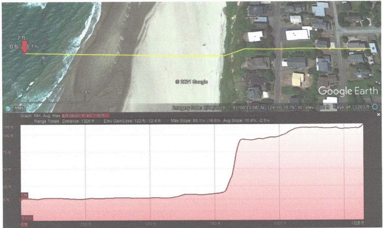
Figure 1: Slopes at the subject site, as presented by Google Earth.
