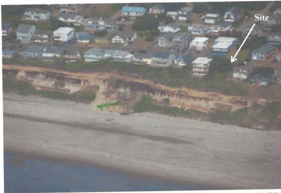
Figure 2: Image of the subject site and adjacent parcels, excerpt from O-15-06. Original caption read: Oblique aerial photo of homes perched along the cliff top at Roads End, Lincoln City, Oregon. Dark banding in the upper terrace face reflects ground water seepage down through the terrace sediments, where it comes in contact with the less permeable tertiary siltstones of the Yamhill Formation. Note the recent slump failure in mid photo (photo: E, Harris, DOGAMI, 2011).
