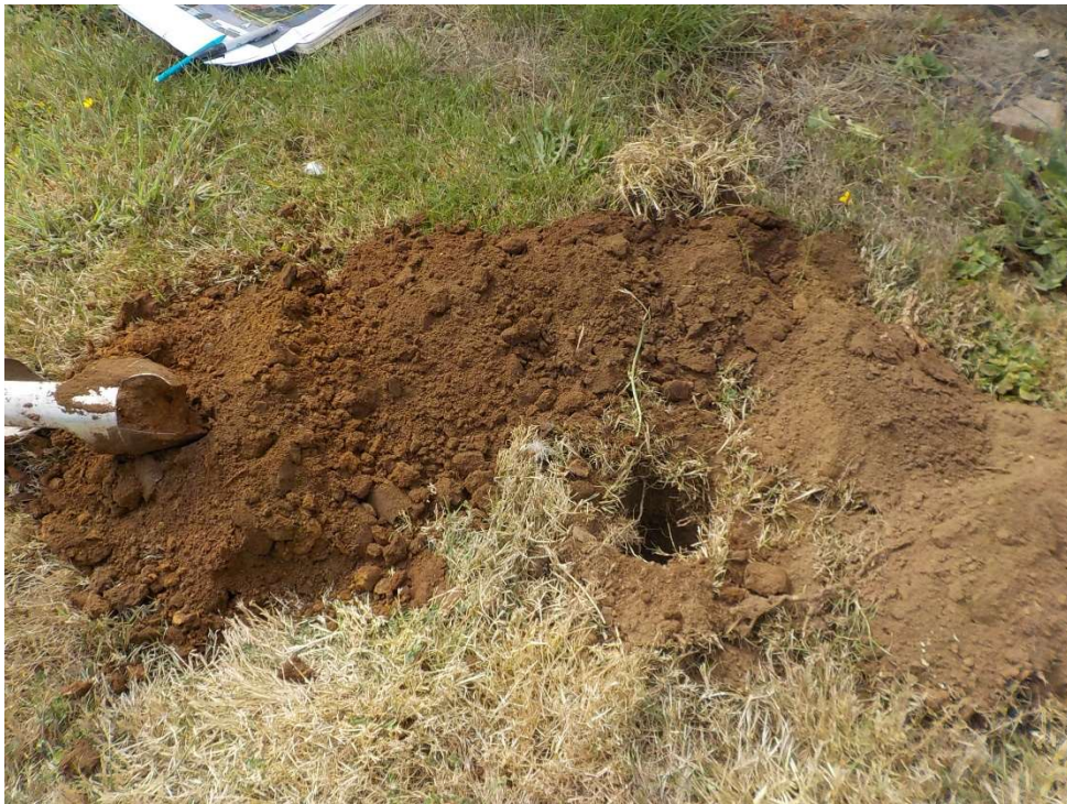
Photo 6 – View of the soils encountered in Boring B-2.
