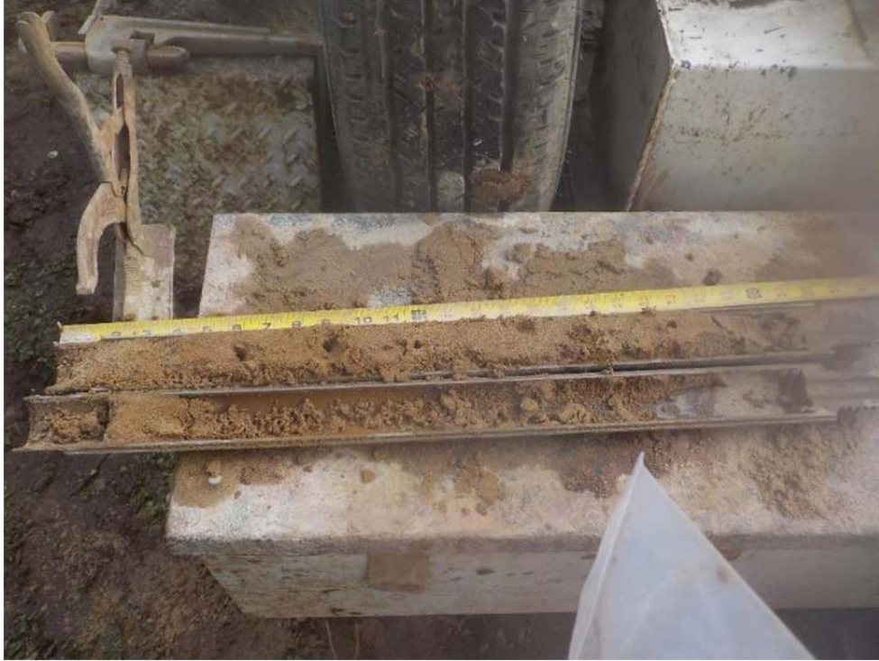
Photo 17 – Close-up view of the native dense sands typical of that recovered in the boring (4/12/2018).
