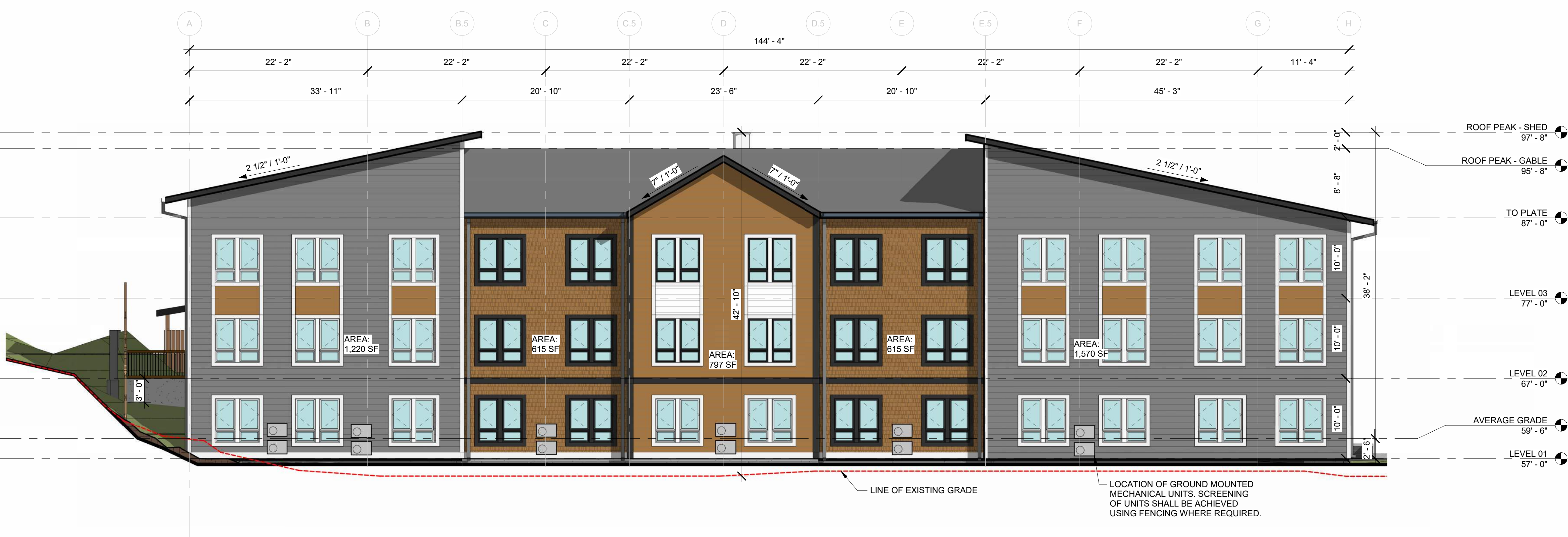
2 EXTERIOR - REAR WEST ELEVATION 1/8" = 1'-0"
