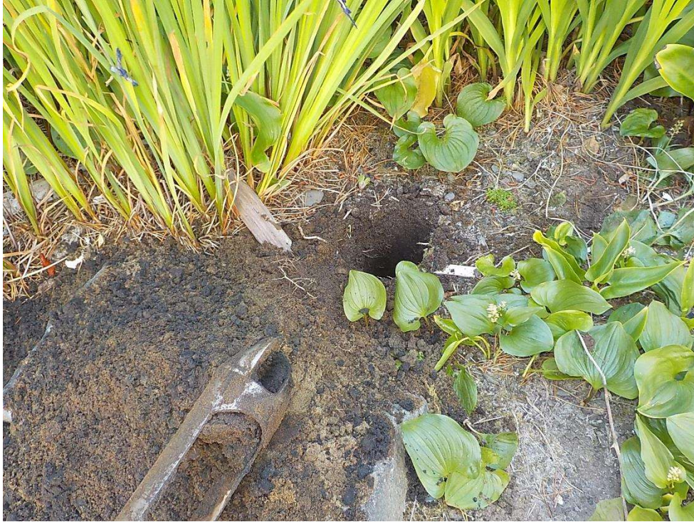
Photo 7 – Close-up view of the fill and loose sandy soils encountered in boring B-1.
