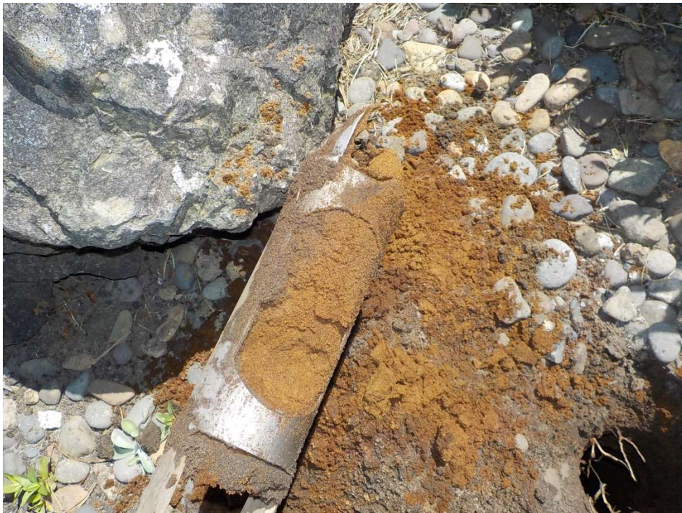
Photo 8 – Close-up view of medium-dense sandy soils encountered in boring B-2.
