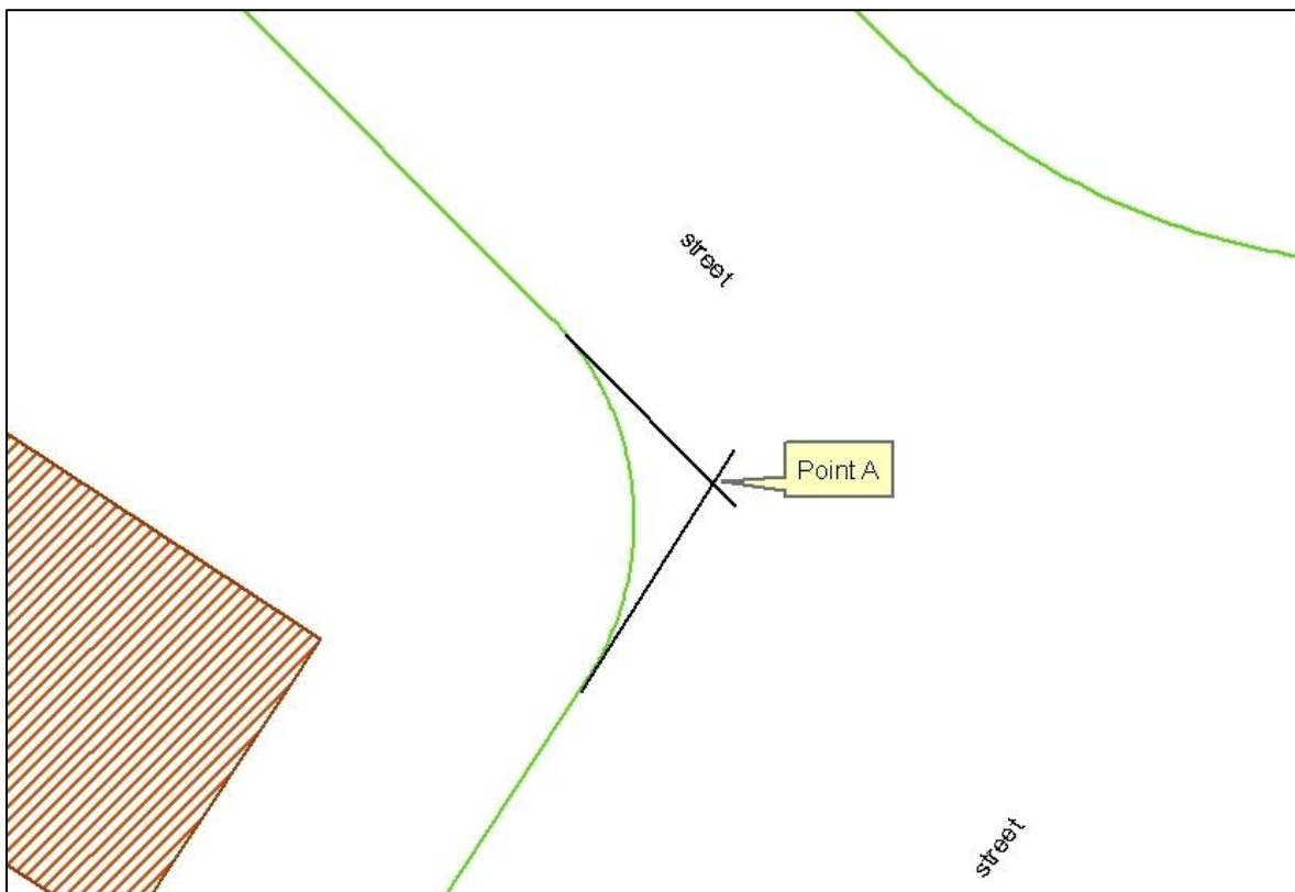
Figure 17.52.060-3: Clear-vision triangles at uncontrolled intersection.
